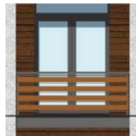
4 STEEL CABLE RAILING W/ BOARD
