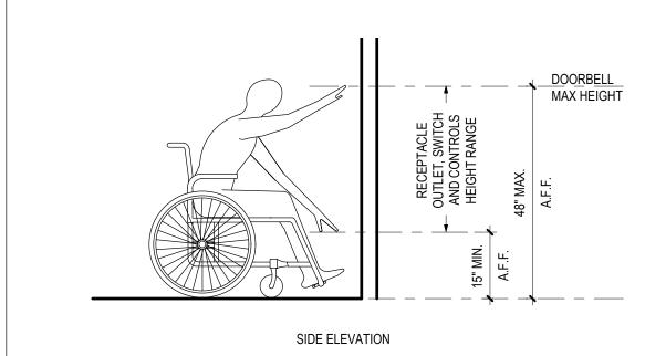
R327.1.2 ELECTRICAL RECEPTACLE OUTLET, SWITCH AND CONTROL HEIGHTS & R327.1.4 DOORBELL BUTTONS
