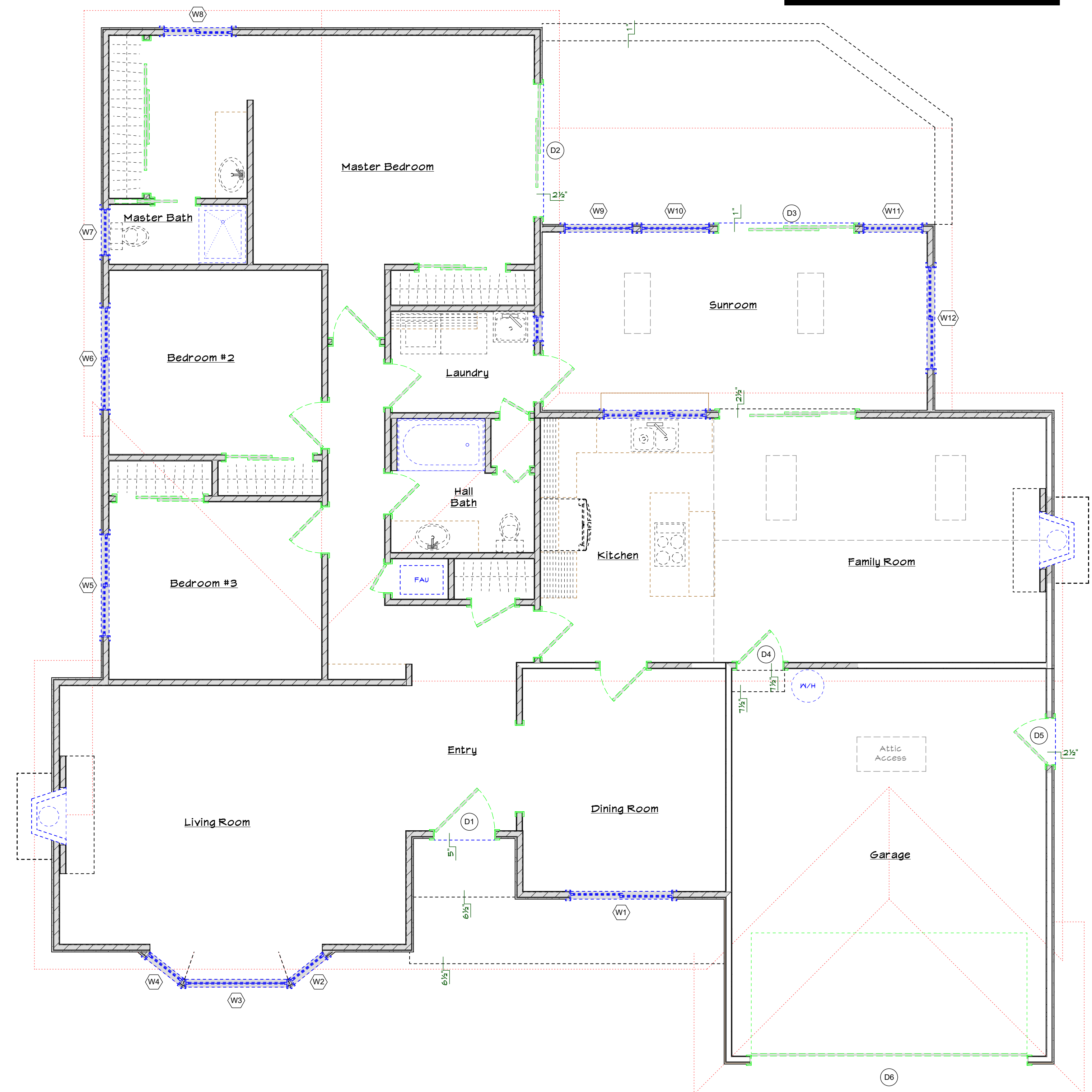
EXISTING/DEMOLITION FLOOR PLAN Scale: 1/4" = 1'-0"
