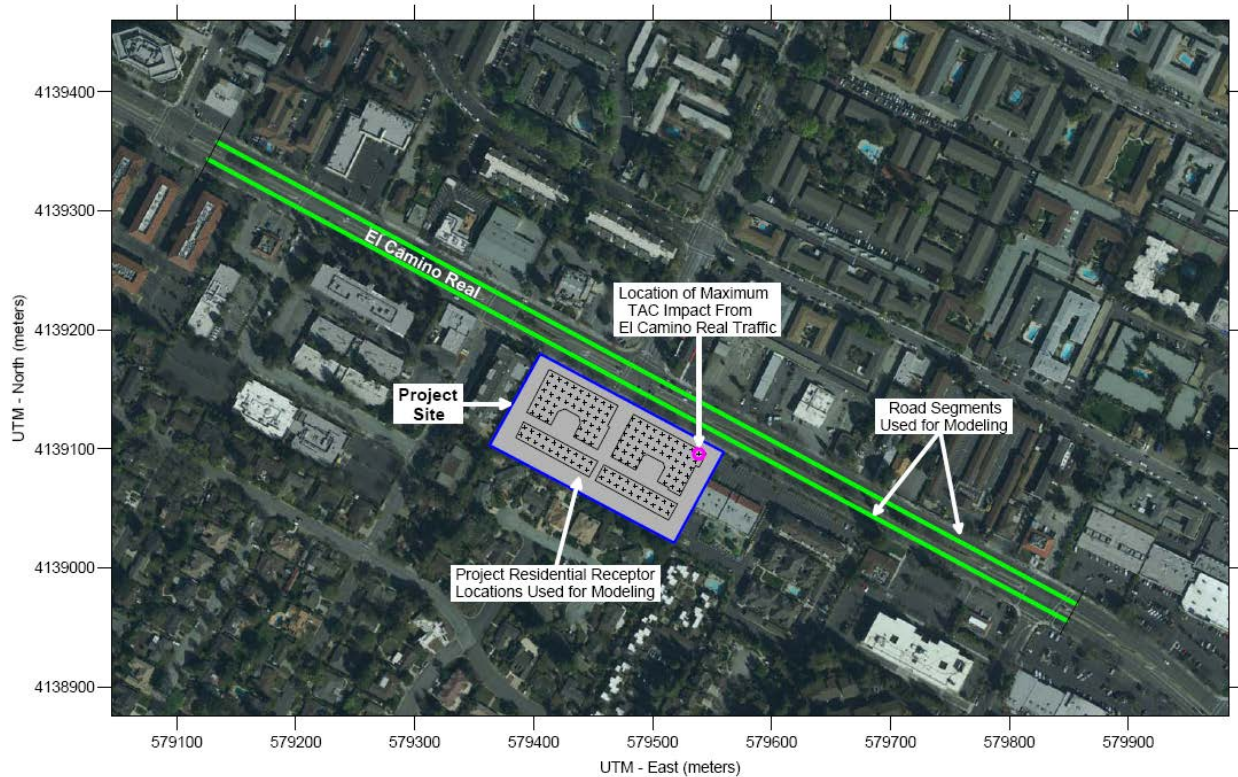
Figure 3. Project Site, On-Site Sensitive Receptors, Roadway Segments Modeled and Receptors with Maximum TAC Impacts
