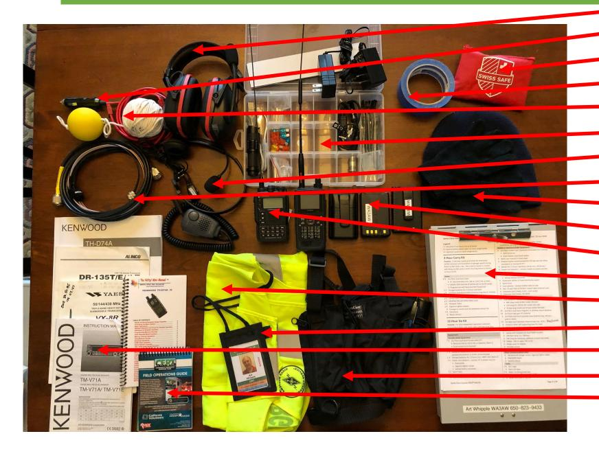
Headset – stationary 12V auto supply First aid kit Tape Ball and string Connectors/stuff Headset - mobile Hang-up J-pole antenna Warm hat and gloves Spare charged batteries 2 hand-held transceivers Closed clipboard Vest Los Altos DSW badge **Equipment manuals** Radio chest pack
