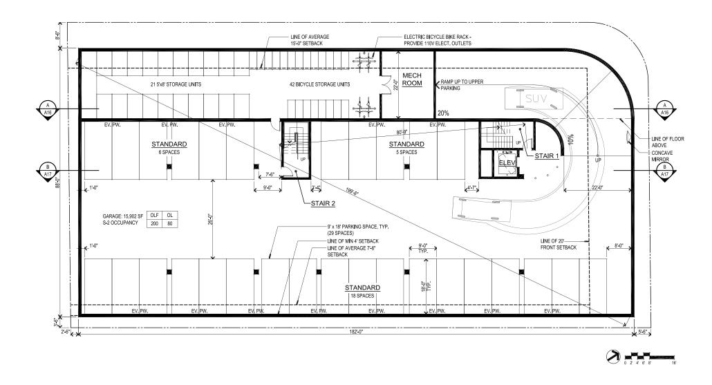
Figure 7A Lower Level Basement Turning Movements
