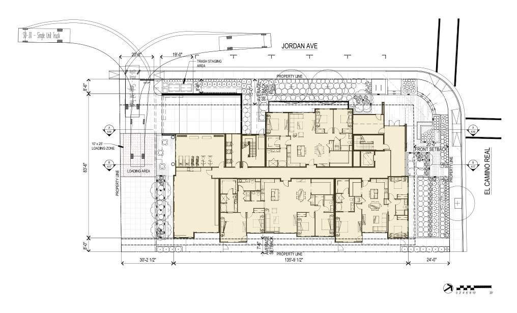
Figure 8 Loading Zone Turning Movement
