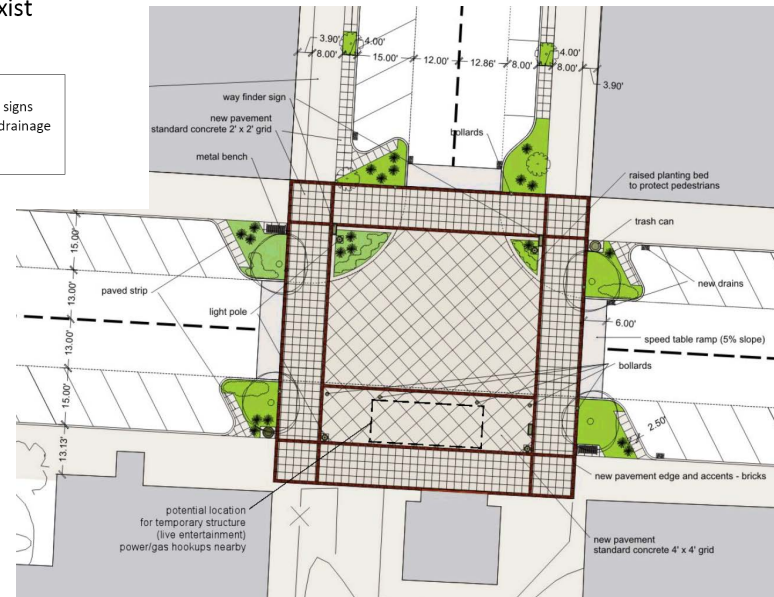
Figure 12. Suggested intersection and traffic calming design on First Street.
