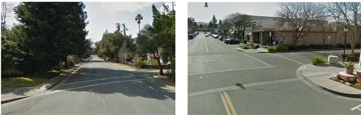
Figure 3-16: Example of a minimal crosswalk treatment across Edith Avenue at 4th Street (left), and a decorative crosswalk with curb extensions on Main Street in downtown Los Altos (right)
