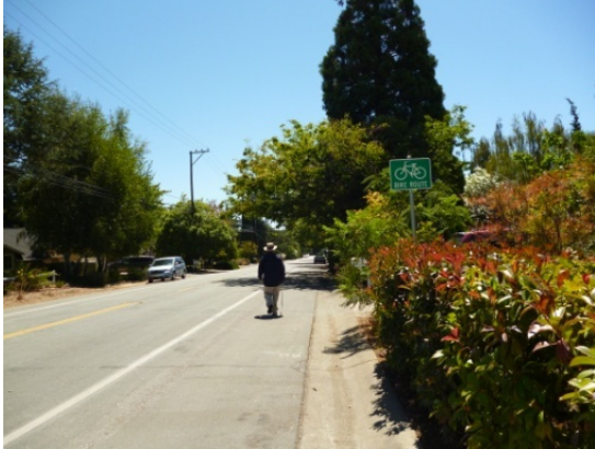
Figure 3-11: Paved shoulders often double as parking lanes, sidewalks, and bicycle facilities in many residential neighborhoods in Los Altos(left). An asphalt berm (right) converts a paved shoulder into an informal walkway.
