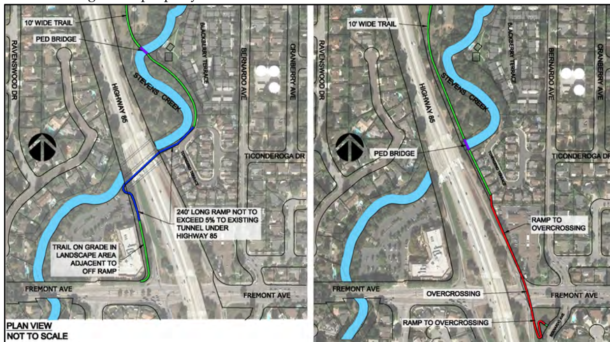
Figure 24 – Grade-separated options for connecting to Fremont Avenue.
