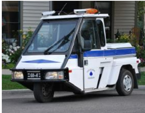
Figure 2-4 Mobile License Plate Recognition on Enforcement Vehicle 19
